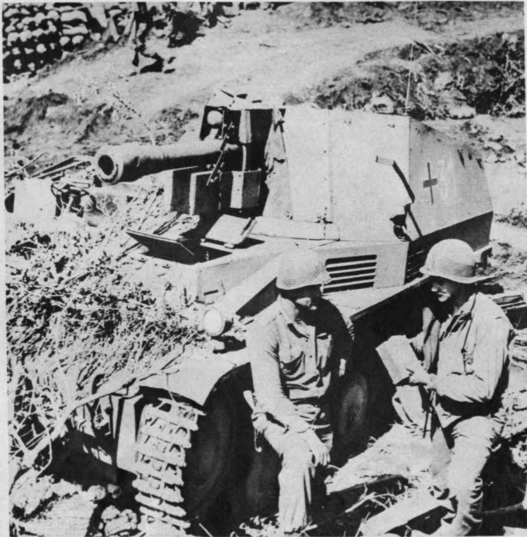
Wasp mounting a 105-mm. light field howitzer is the only one of the Insect series that does not incorporate the PzKw IV chassis. Packing blocks around the gun buffer suggest this Wasp never had time to fire a shot. From it American troops in Italy carefully remove a booby trap.
